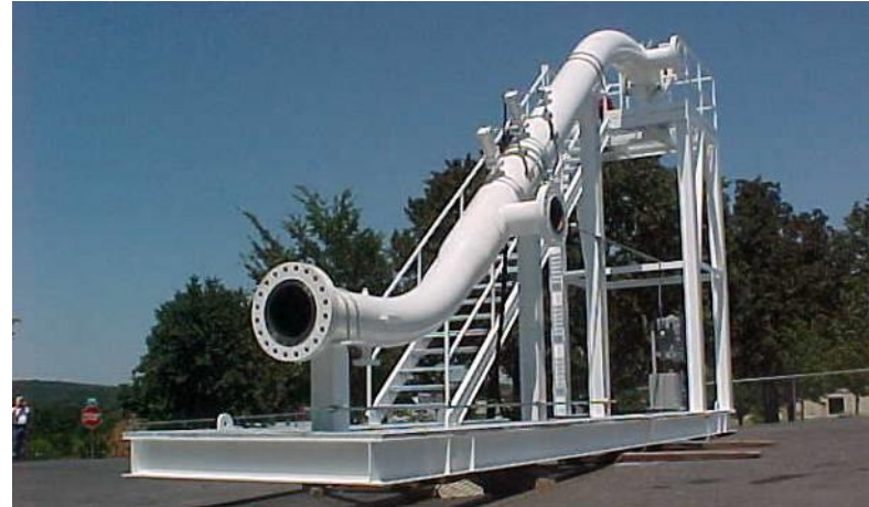
Weekly scraping (via remote operated multi scraper launcher)
